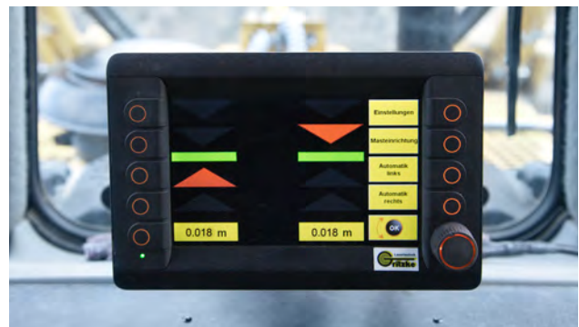
Figure 2: Working surface with following setting options: "Mast installation" e.g. "search laser" or "park mast", automatic mode for the right or the left mast "on / off", "mast adjustment on both sides", as well as current height indication in 1/10 mm (Photo: ifm)
