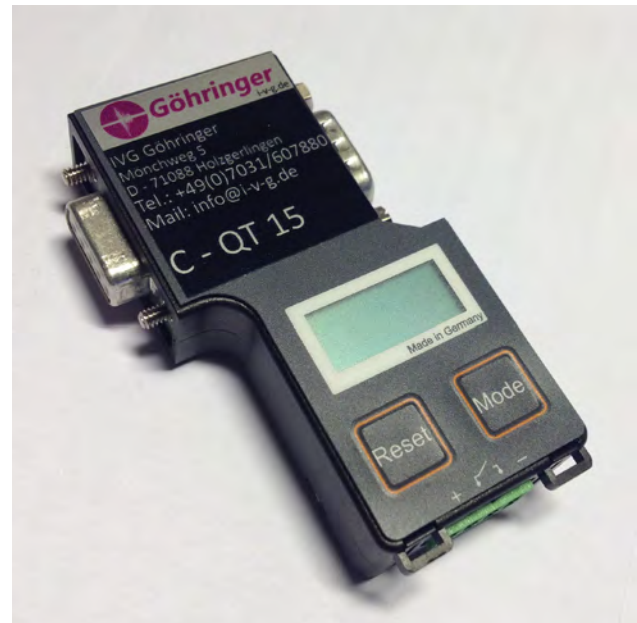
Figure 1: Errors in CAN communication are indicated by the integrated status LEDs and a potential-free alarm contact (Photo: IVG Göhringer)
