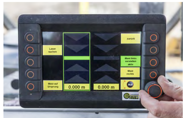
Figure 6: The CR1084 dialog monitor from ifm Electronic for visualization and data entry (Photo: ifm)
