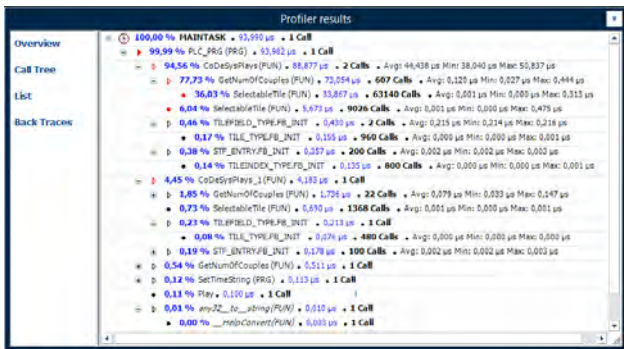
Figure 4: Time analysis on the device with Codesys Profiler (Photo: 3S)
