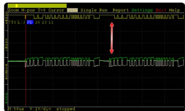
Figure 3: The upper curve displays the data stream from the CAN transceiver; the marked position exemplarily shows that the transceivers threshold is not reached by the analog signal (Photo: Peak-System)
