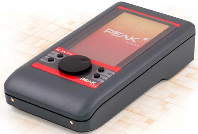
Figure 2: Handheld device PCAN-Diag FD for diagnosis of a CAN FD network (Photo: Peak-System)
