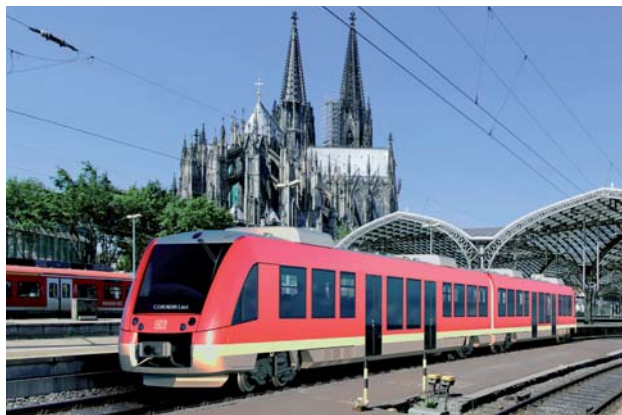
Figure 2: Three MTU Powerpacks will power Alstom's Coradia Lint 54 diesel railcars operating in the Cologne Diesel Network
