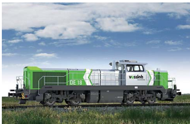
The DE 18 four-axle diesel-hydraulic locomotives by Vossloh provide an automatic start-stop eco drive system, slip protection, and driver assistance
